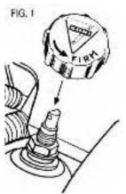
These shocks do not need to be removed from the vehicle to be adjusted. Please the adjustment knob included with the shocks onto the adjuster tab on the top of the shock absorber. Turn the adjusting knob clockwise to check if the damper has been previously adjusted. If you feel resistance, DO NOT FORCE, as the shock is in the minimum position.
