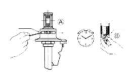
The Rebound adjuster requires a pin with an outside diameter of 3mm or a 2.5mm hex key. To increase the rebound force, put the adjuster pin in the hole next to the minus sign and turn the pin towards the plus sign. This is one sweep of adjustment. The total adjustment range is 7 to 8 sweeps. There are no specific clicks to mark the adjustment position; the rebound adjuster can be placed in any position in the adjustment range.
