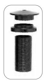
The threaded sleeves are designed to mount on fixed platforms or groove located circlips that are perpendicular to the damper body. The threaded sleeves are made of anodized aluminum with threading specially designed for load carrying and self cleaning properties. All lower perches have a nylon tipped locking set screw to positively lock the perch in place without damaging the threads.
