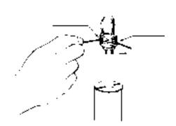
The rebound and compression adjuster requires a pin with an outside diameter of 1.5mm or a 1.5mm hex key. The adjusters are marked with the letters that are stamped on the mounting eye.
